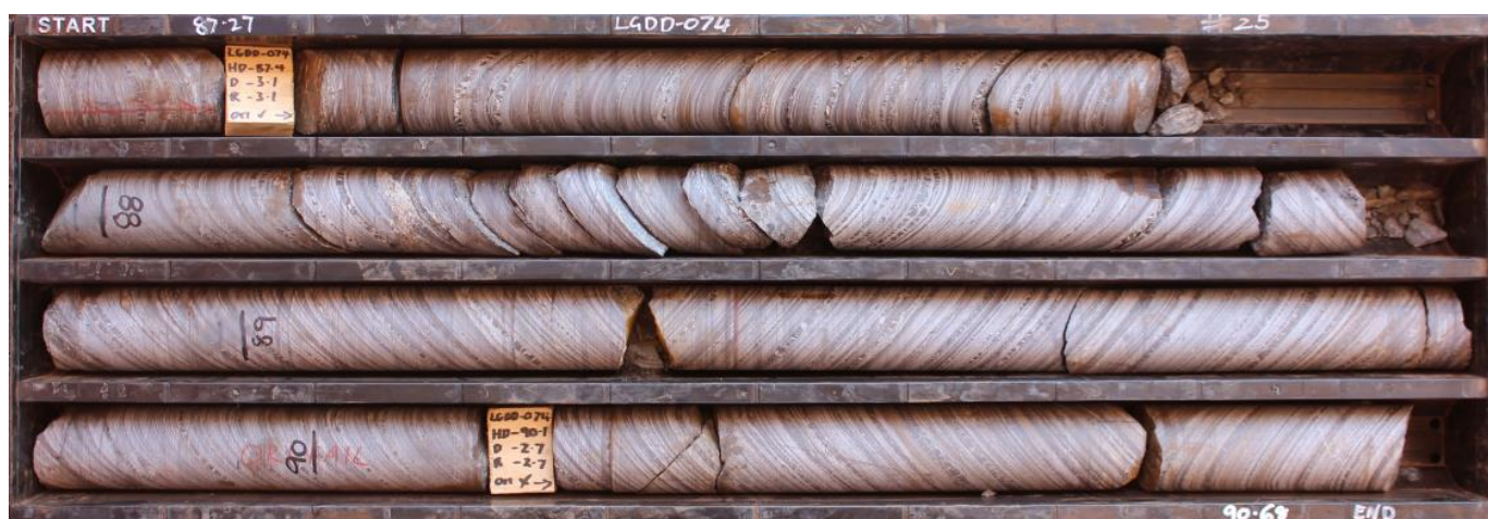
Photo 1 - Strong magnetite mineralisation at Moonshine North Zone in diamond drill hole LGDD_074
