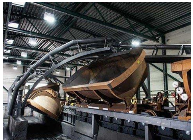
Conceptual example of ‘Helix Dumper’ in operation. Image is not a representation of actual infrastructure at the Port of Esperance. (Image reproduced with permission from Kiruna Wagon and RCR MT)
