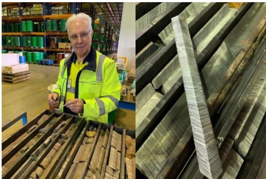
Figures: Sample inspection of Macarthur's magnetite core by Stantec's Mr Neville Dowson
