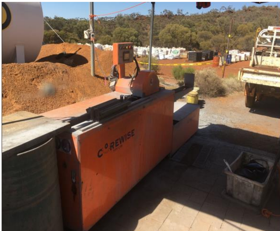
Figure 11-3: Diamond saw used for cutting diamond core, as used during the 2019 drilling program
