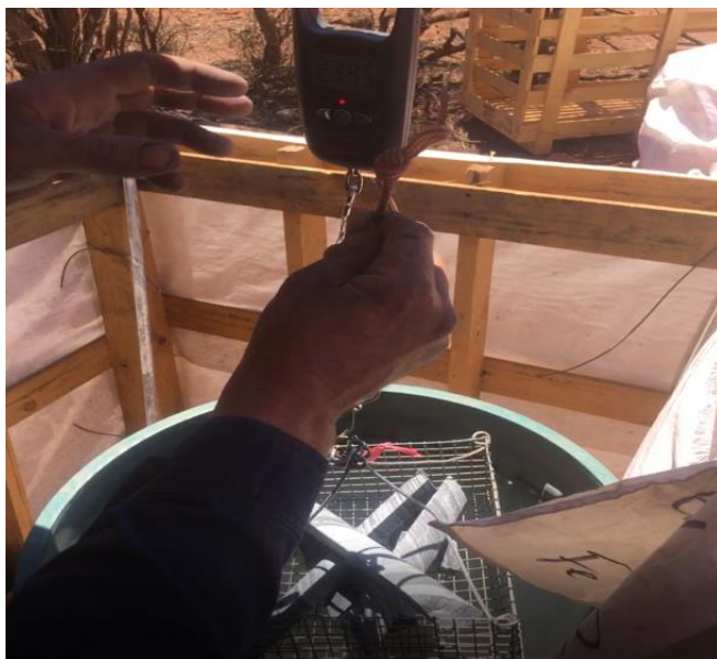
Figure 10-5: Dry Core Samples Prior to Immersion and Weighing in Water
