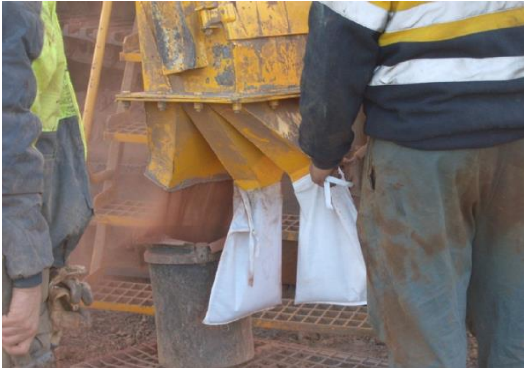
Figure 11-1: Three-tiered splitter on an RC drill rig, showing collection of primary sample and field duplicate (sample residue is collected in the bucket)
