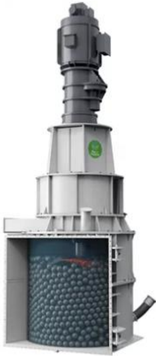
Figure 17-6: Cutaway View of Vertimill®
